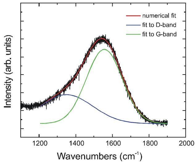
Fig. 2 Raman spectra of sample 51001a, fitted with two Gaussian peaks for the G- and D-mode
