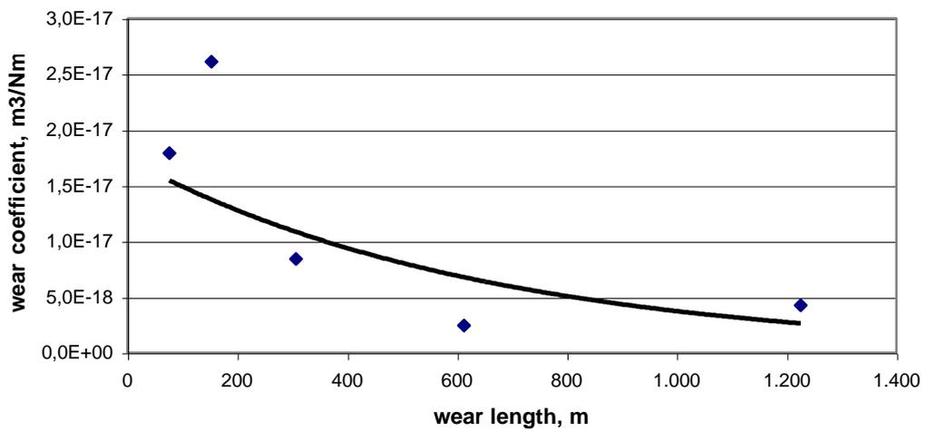
Fig. 1 Wear coefficients of a series of ball craters on sample 51001a corresponding to the wear length
