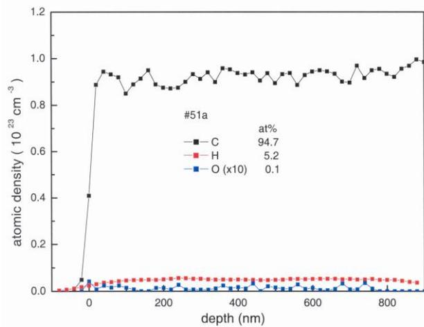
Fig. 3 ERDA-based depth profile of sample 51001a
