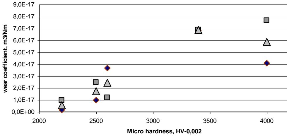
Fig. 4 Wear coefficients of a series of the samples depend on the micro hardness values
